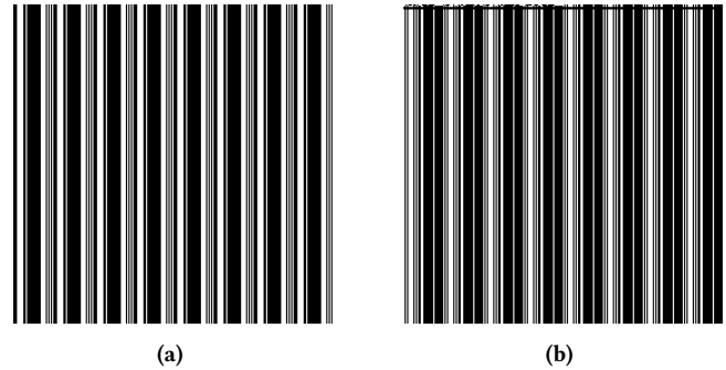
Figure 7: Snapshots of i-cache after attacking bare-metal software in (a) BCM2711 and (b) BCM2837 SoCs. Uninitialized cache cells power on into random state (see Figure 3), but when we execute Volt Boot attack, instructions stay in the i-cache across power cycles.
